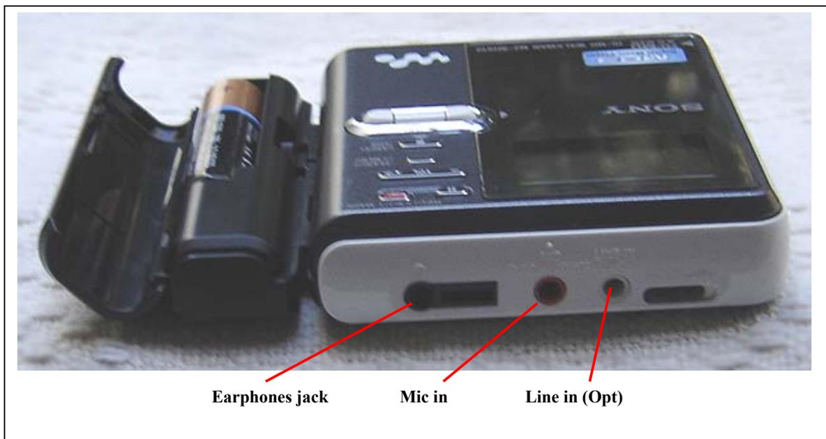
A) The audio-recorder device used is a Sony Hi-MD, Model No. MZ-RH910 (similar models: MZ-RH1; MZ-M200) which has the following inputs and outputs:
